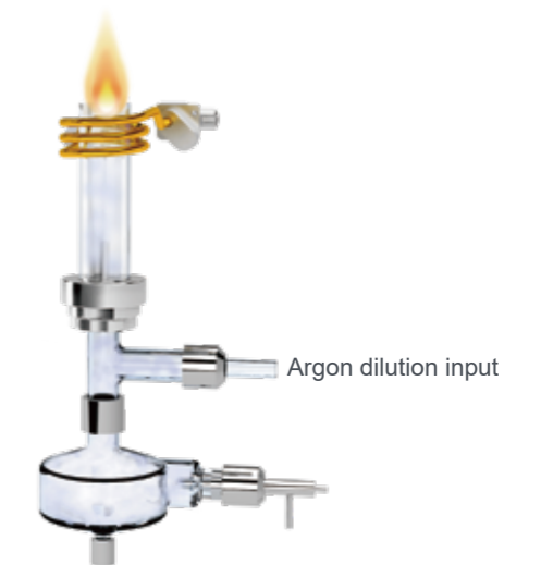
Schematic diagram for argon dilution input
